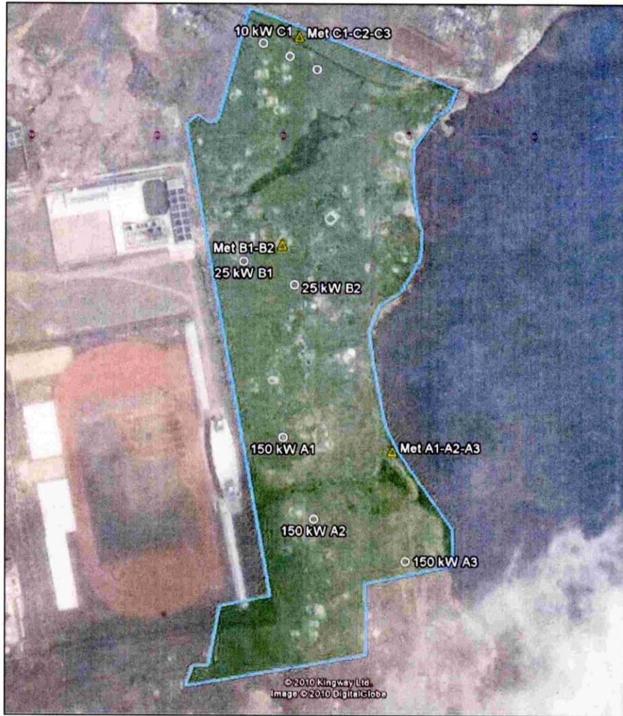
Figure 2-1. Map of the TERTEC Test Site, Layout A
